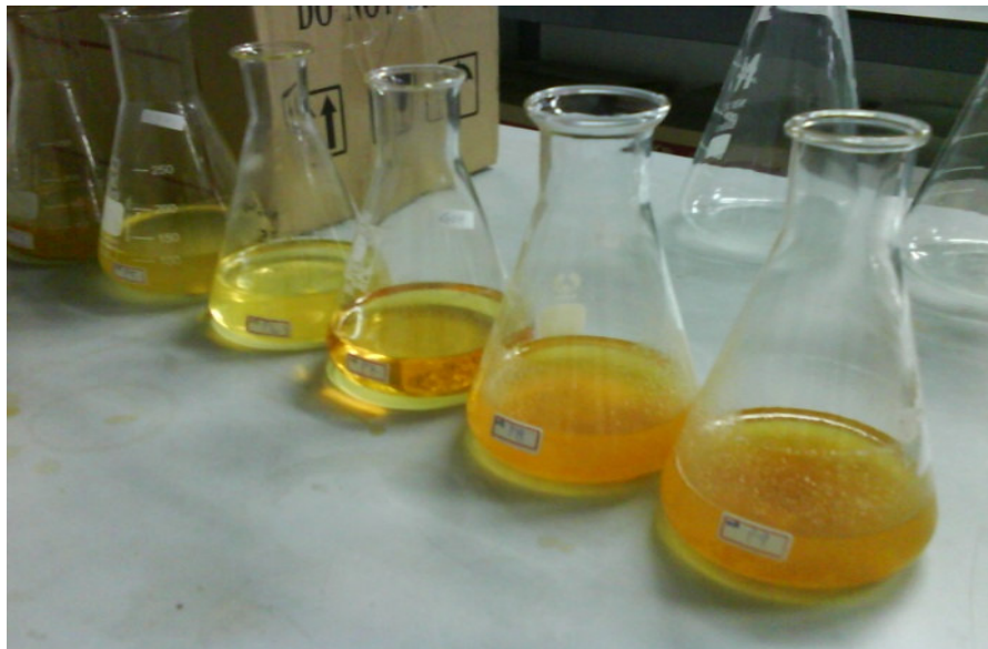
Figure 6. Biodiesel produced from waste soybean oil. Lower layer indicates glycerin and upper layer indicates biodiesel ester..
