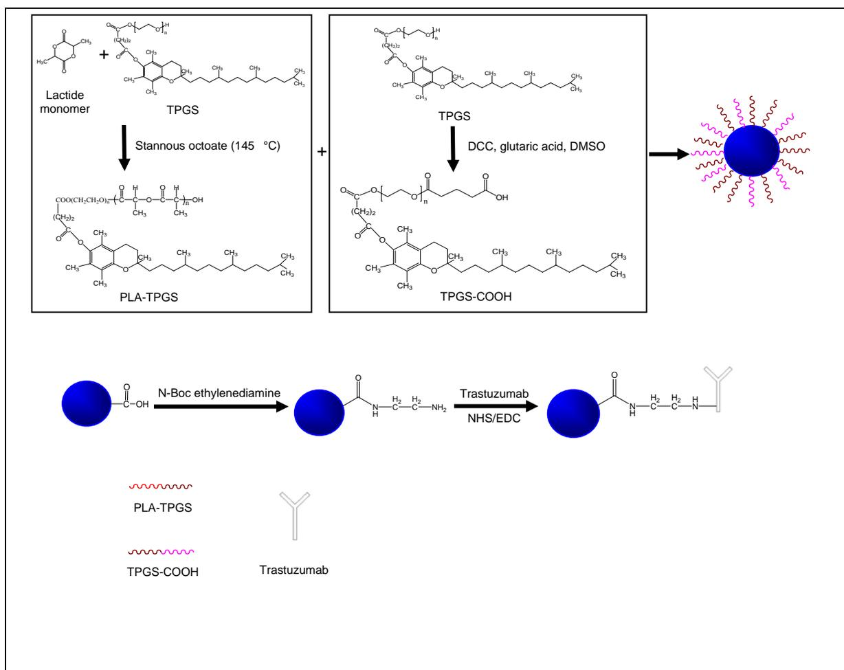
**Figure 2. Schematic illustration for preparation of the Trastuzumab-functionalized, Docetaxel-loaded PLA-TPGS/TPGS-COOH nanoparticles.**
