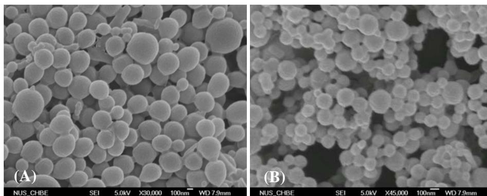
**Figure 1. Field Emission Scanning Electron Microscope (FESEM) images of PLGA nanoparticles fabricated by (A) the solvent extraction/evaporation method; and (B) the nanoprecipitation method.**
