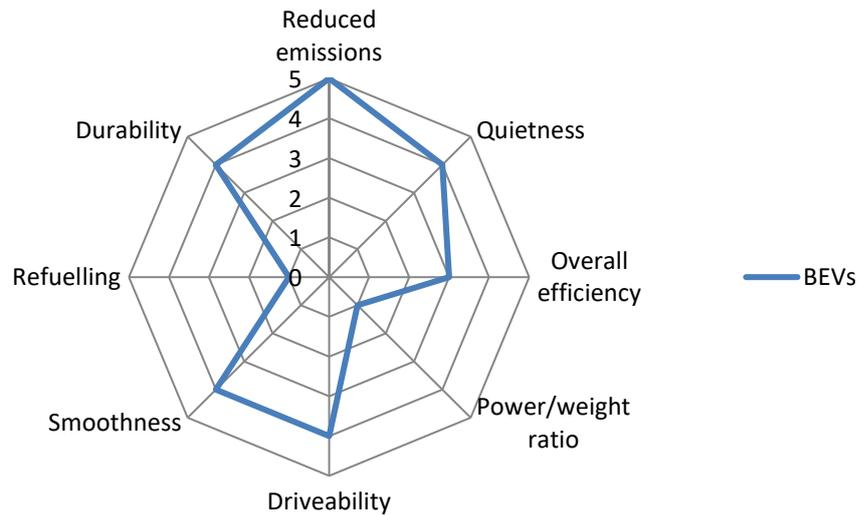
**Figure 1.2** Relative comparison of advantages and disadvantages of BEVs over ICEVs [3]
