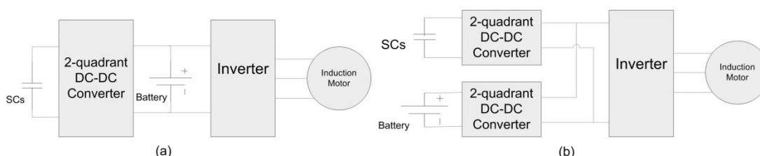
**Figure 1.4** Connection scheme of HESS (a) single converter scheme and (b) multiple converter scheme
