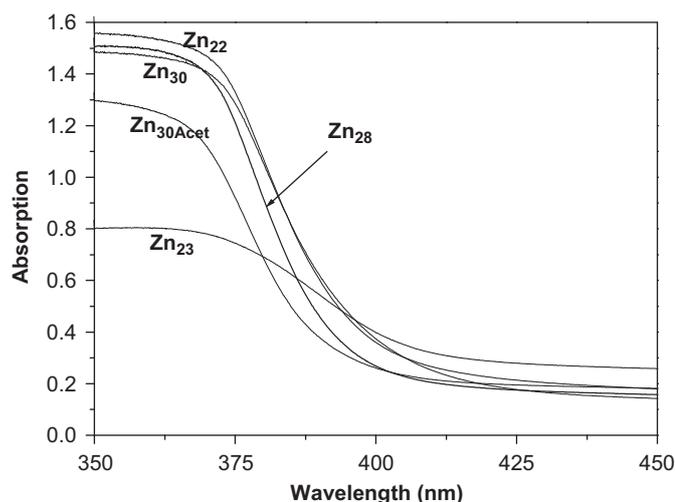
**Fig. 10.** UV-vis absorption spectra of ZnO particles with different morphologies: nanorods (sample Zn<sub>22</sub>), irregular morphology (sample Zn<sub>23</sub>), conical morphology (sample Zn<sub>28</sub>), spherical morphology (sample Zn<sub>30</sub>) and rod-like morphology (sample Zn<sub>30Acet</sub>).
