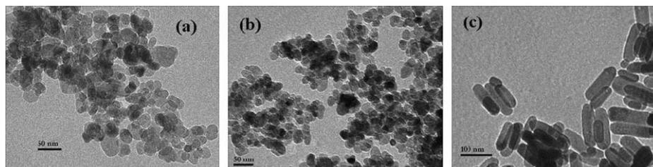
**Fig. 2.** Transmission electron microscopy images of ZnO nanoparticles grown at 100 °C (a) 180 °C (b) and 245 °C (c).
