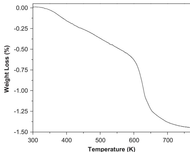
Fig. 9. TG curve of the conical particles from RT to 773 K.
