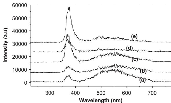
**Fig. 11.** Room-temperature photoluminescence (PL) spectra of ZnO particles presenting different morphologies: nanorods (a), spherical morphology (b), conical morphology (c), irregular morphology (d) and rod-like morphology (e).
