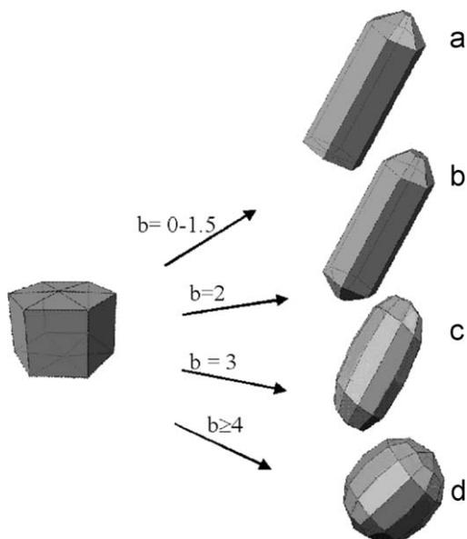
Fig. 8. Evolution of the ZnO particles morphology as a function of the alkaline ratio.
