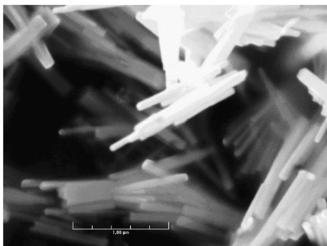
Fig. 5. SEM micrograph of the  $\text{Zn}_{30\text{acet}}$  powder.
