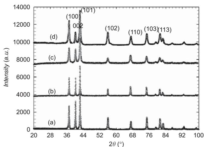
Fig. 1. Powder X-ray diffraction patterns of the as-synthesized ZnO (a) conical particles, (b) nanorods, (c) spherical particles and (d) rod-like particles.
