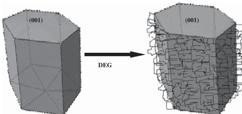
Fig. 6. A schematic view of showing the primary particles of ZnO with the DEG molecules adsorbed on its non-polar faces.
