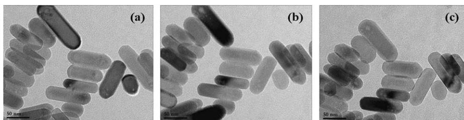
Fig. 3. Transmission electron microscopy micrographs of the ZnO nanorods obtained at different tilt positions (a)  $x = 0$ , (b)  $x = 20$  and (c)  $x = 30$ .
