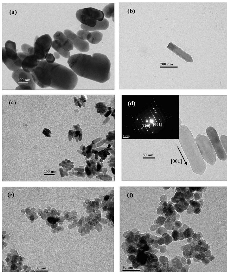
Fig. 4. TEM micrographs of ZnO nanopowder obtained at different alkaline ratios (a)  $b = 0$ , (b)  $b = 0.5$ , (c)  $b = 1.5$  and (d)  $b = 2$ , within inset the SAED pattern on one nanorod, (e)  $b = 3$ , (f)  $b = 4$ .
