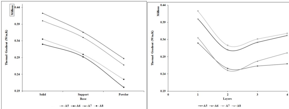
Figure 3: Thermal gradient (a) at different bases in the first layer, and (b) along the layers on a solid base
